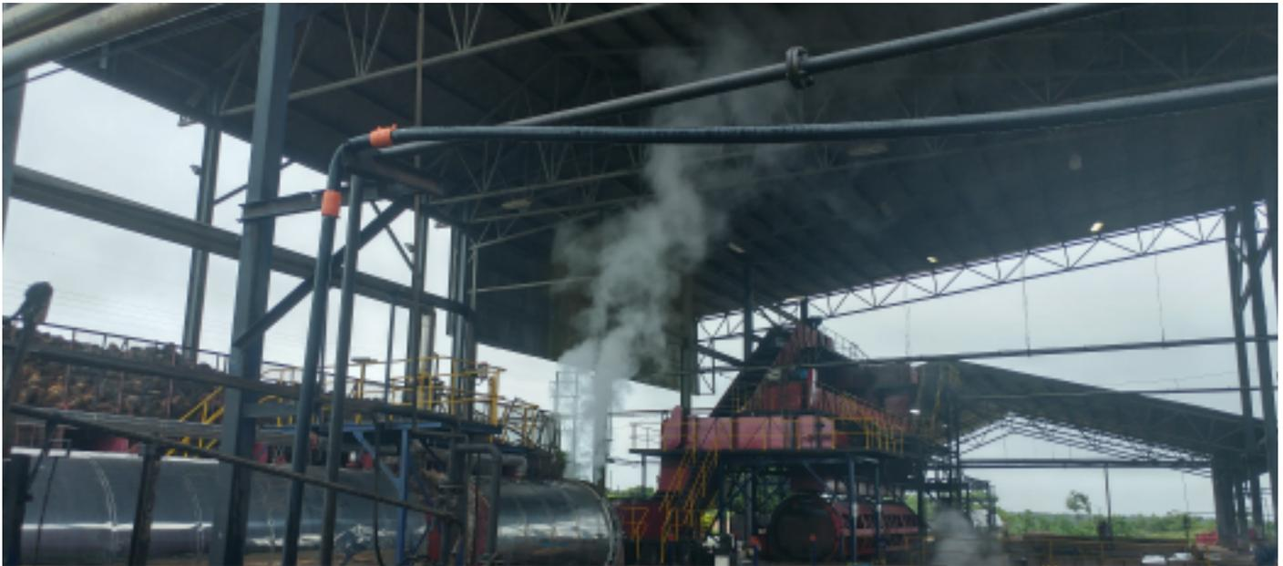
Transport of palm oil slurry at 95°C.
