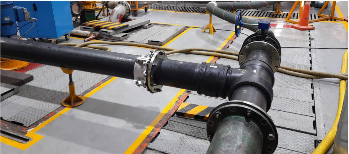
Replacement of steel pipes with Pexgol for testing centrifugal pumps.
